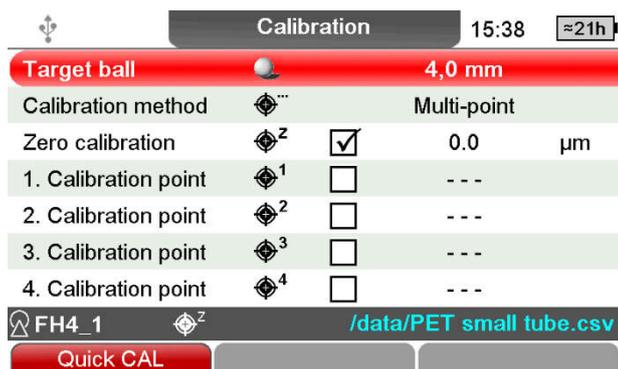
MiniTest FH uses AI to detect the diameter of the measuring ball inserted in the zero cap and automatically performs a zero calibration for this ball diameter.
