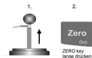
Hold the sensor in the air and press ZERO/∞ key for several seconds.
