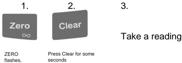
Calibration using a calibration foil. Recommended if the test sample is coated and no uncoated sample is available for comparison. This method is suitable for the following probes.
