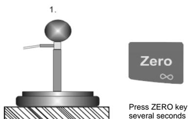
Place the sensor on the coating material (min. 30 mm) avoiding any metal support!
