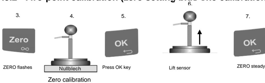
Press the ZERO key and place the sensor on the zero standard. Press the OK key shortly several times, the mean value of readings is calculated. Lift the sensor and press OK key shortly.
