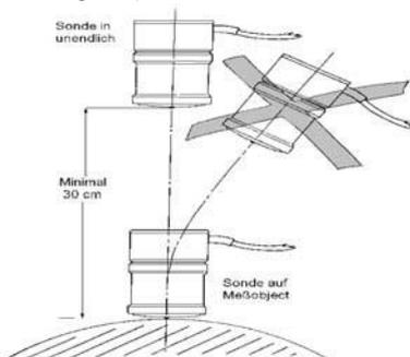
In order to avoid hysteresis errors, after each measurement, the probe must be held away from the measuring object ensuring a minimum distance of 0.3m / 12“ away from any metal parts.
