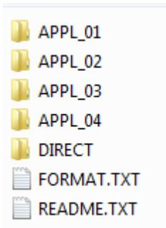
The application memories (APPL) with their corresponding batch memories (BATCH) allow to store calibration settings for different applications in an application memory (APPL). The batch memory (BATCH) stores single readings of a series of measurement along with their statistical analysis (see illustration: APPL-BATCH memory).
