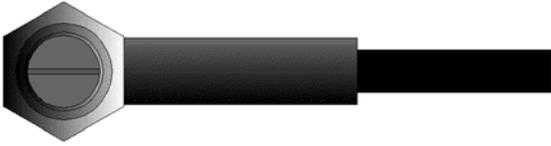
This is a bottom view of a typical transducer. The two semicircles of the wearface are visible, as is the barrier separating them
