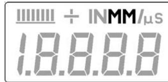
When the **MM** symbol is on, the *MiniTest 405* is displaying a thickness value in millimeters. If the displayed thickness exceeds 199.99 millimeters, the decimal point will shift automatically to the right, allowing values up to 1999.9 millimeters to be displayed.
