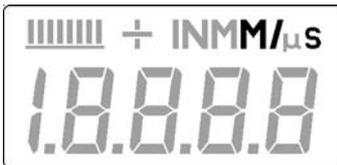
When the **M** symbol is on, in conjunction with the **/s** symbol, the **MiniTest 405** is displaying a sound-velocity value in **meters-per-second**
