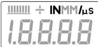
When the **IN** symbol is on, in conjunction with the **/μs** symbol, the **MiniTest 405** is displaying a sound-velocity value in **inches-per-microsecond**
