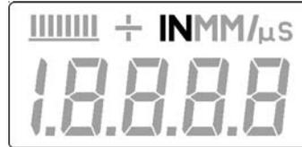
When the **IN** symbol is on, the *MiniTest 405* is displaying a thickness value in inches. The maximum thickness that can be displayed is 19.999
