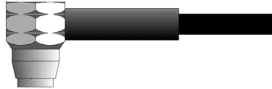
The transducer is the „business end“ of the **MiniTest 405**. It transmits and receives ultrasonic sound waves that the **MiniTest 405** uses to calculate the thickness of the material being measured. The transducer connects to the **MiniTest 405** via the attached cable, and two coaxial connectors. When using transducers manufactured by ElektroPhysik, the orientation of the dual coaxial connectors is not critical: either plug may be fitted to either socket in the **MiniTest 405**.
