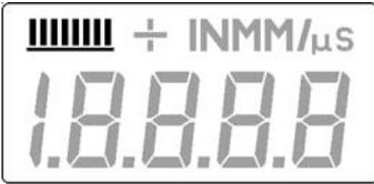
These eight vertical bars form the Stability Indicator. When the *MiniTest 405* is idle, only the left-most bar and the underline will be on. While the gauge is taking a measurement, six or seven of the bars should be on.
