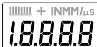
The numeric portion of the display consists of 4 complete digits preceded by a leading „1“, and is used to display numeric values, as well as occasional simple words, to indicate the status of various settings.
