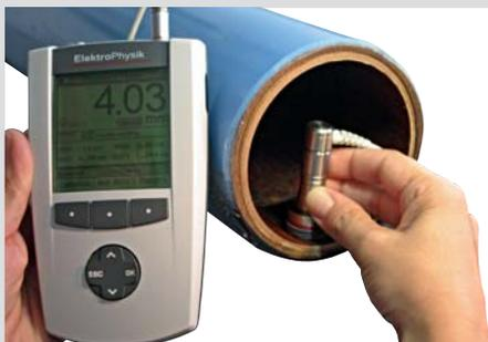
Harsh environments or contamination through paint or dust particles require specially adapted sensors. To provide the ultimate protection to your harsh environment demands, the MiniTest 7400 line offers a special range of rugged sensors (HD sensors). These sensors feature a special grout sealing to protect the sensor electronics. An external spring mounting system is provided to ease sensor cleaning.
