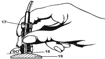
17 Spring-mounted sleeve for holding the probe
