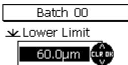
Tolerance limits can be set at any time before, during or after acquisition of readings.
