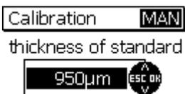
Press OK to store the calibration point. Press OK once again to complete the calibration procedure.
