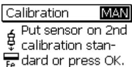
Put the second precision standard on the uncoated calibration sample. Place the sensor on top of it, wait for the signal to sound and lift sensor. Repeat this procedure several times (approx. 3 to 10 times) on the same measuring spot. The average  $\bar{x}$  will be shown.
