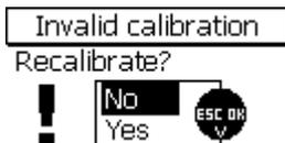
With all predefined calibration methods (except for "Factory" and "Manual") the following message will appear once you have run through the batch creation procedure: "Invalid calibration – recalibrate?". At this point you can decide whether to recalibrate immediately or at a later point in measure mode.
