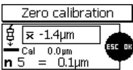
Repeat this procedure several times (approx. 3 to 10 times) on the same measuring spot. The average  $\bar{x}$  will be shown. Evaluation of average is to increase accuracy of calibration. Accuracy will increase with an increasing number of readings. Press OK to confirm the calibration point. Press OK once again to complete the calibration procedure.
