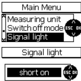
The gauge features a signal light (above the MENU key) to indicate whether a reading is within tolerance (green light) or beyond tolerance (red light). The duration of light signal can be adjusted to “short on”, “off” or “long on”.
