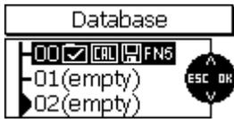
Use arrow up/down keys to select an “empty” batch. Press OK to confirm. The selected batch will open.
