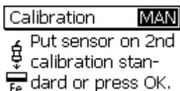
Put the second precision standard on the uncoated calibration sample. Place the sensor on top of it, wait for the signal to sound and lift sensor. Repeat this procedure several times (approx. 3 to 10 times) on the same measuring spot. The average  $\bar{x}$  will be shown.
