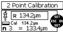
If the shown set point (Cal) as displayed is not identical with the thickness of your precision standard, use arrow up and down keys to adjust accordingly.
