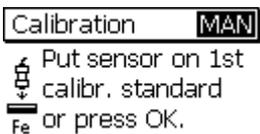
Put the first precision standard on the uncoated calibration sample. Place the sensor on top of it, wait for the signal to sound and lift sensor. Repeat this procedure several times (approx. 3 to 10 times) on the same measuring spot. The average  $\bar{x}$  will be shown.
