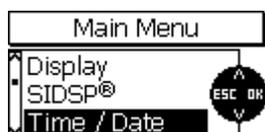
The gauge features a quartz-controlled time clock to indicate date and time. The current time is shown top right in the status line (visible in measuring mode only). The time clock is also used for fixing date and time of creation / last modification of a batch. Date and time of creation/ last modification will also be stored and indicated with a batch and displayed while opening this batch.
