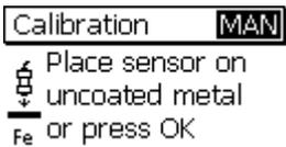
Start calibration and put the sensor on the blank/uncoated calibration sample. Wait for the signal to sound and lift sensor. Please observe the instructions in section 6.1 General.
