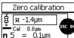
Repeat this procedure several times (approx. 3 to 10 times) on the same measuring spot. The average  $\bar{x}$  will be shown. Evaluation of average is to increase accuracy of calibration. Accuracy will increase with an increasing number of readings. Press OK to confirm zero calibration. Press OK once again to complete the calibration procedure.
