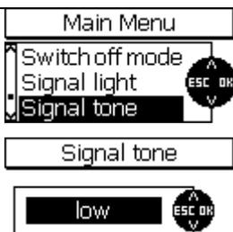
The signal tone is to confirm acquisition of readings and to confirm key action.
