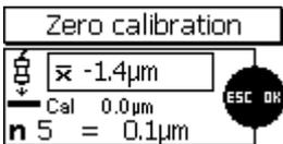
Repeat this procedure several times (approx. 3 to 10 times) on the same measuring spot. The average  $\bar{x}$  will be shown. Evaluation of average is to increase accuracy of calibration. Accuracy will increase with an increasing number of readings. Press OK to confirm zero calibration. Press OK once again to complete the calibration procedure.
