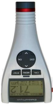
In the measuring mode you can rotate the display by 180°. Press the arrow up/down keys to rotate.
