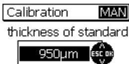
Press OK to confirm the calibration point.
