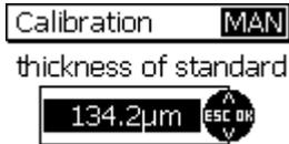
Press OK to confirm the calibration point.
