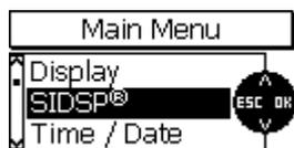
In the SIDSP® menu you can make changes to the measuring mode (normal, fast, high precision).
