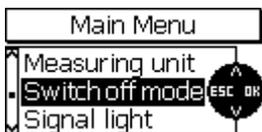
The gauge features a switch-off mode to save battery life. In this mode, the gauge will switch off after the time interval you have fixed if the gauge has been idle for a while.
