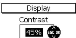
Select „Contrast“ and press OK to confirm. Now use arrow up/down keys to adjust contrast in percent as required (from 30 to 90%). Press OK to confirm your setting.
