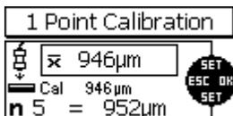
If the shown set point (Cal) as displayed is not identical with the thickness of your precision standard, use arrow up and down keys to adjust accordingly.
