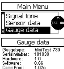
Select “Gauge data” from main menu and press OK to view the gauge specifications. These data should be made available for any service requests.
