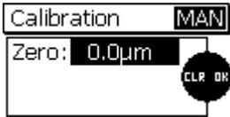
A list will appear to show you the points that have been calibrated. Press OK to go back to the measure mode. In the Auto F/N calibration you will go back to the base selection.
