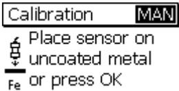
Start calibration and put the sensor on the blank or uncoated calibration sample. Wait for the signal to sound and lift sensor.
