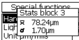
For the single readings statistics, the block size must be adjusted to “1”.
