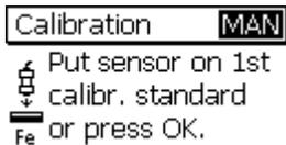
Put the first precision standard on the uncoated calibration sample. Place the sensor on top of it, wait for the signal to sound and lift sensor. Repeat this procedure several times (approx. 3 to 10 times) on the same measuring spot. The average  $\bar{x}$  will be shown. Evaluation of average is to increase accuracy of calibration. Accuracy will increase with an increasing number of readings.
