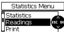
Press function key STAT from measuring mode to call the statistics menu. Use arrow up/down keys to select "Readings" and press OK to confirm.
