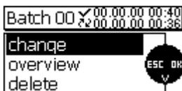
Your selected batch is now active. The display shows name of batch, date and time of batch setting and the last modification. You can select from the following options: change, overview, delete.
