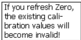
If you have put the sensor on the uncoated sample the message as shown on the left will appear. If during recalibration you refresh zero, you have to repeat all subsequent calibration points.
