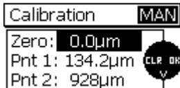
A list will appear to show you the points that have been calibrated. Press OK to go back to the measure mode. In the Auto F/N calibration you will go back to the base selection routine.
