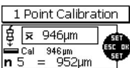
If the set point (Cal) as displayed is not identical with the thickness of your precision standard, use arrow up and down keys to adjust accordingly.
