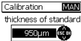
Press OK to confirm the calibration point.
