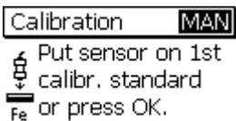
Put a precision standard on the uncoated calibration sample. Place the sensor on top of it, wait for the signal to sound and lift sensor. Repeat this procedure several times (approx. 3 to 10 times) on the same measuring spot. The average  $\bar{x}$  will be shown.
