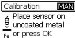
Start calibration. Press OK to jump zero point calibration.
