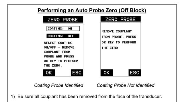
2) Press the **OK** key to perform the automatic probe zero, or **ESC** key to cancel the zero operation.
