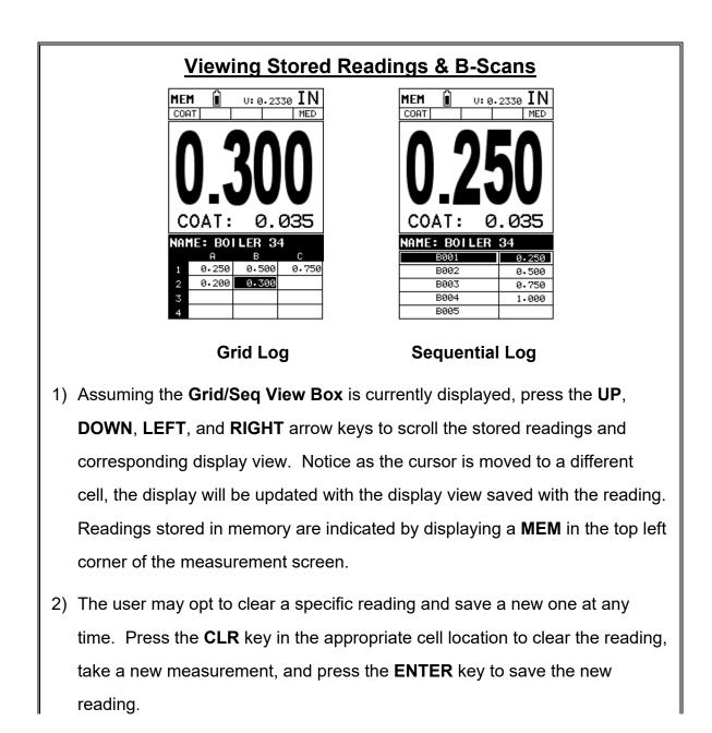
3) Abort the Grid/Seq Log View Box by pressing the MEAS key at any time.
