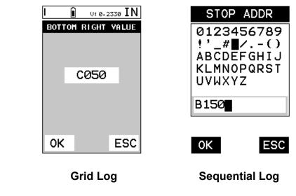
3) <u>**GRID LOG:</u>** Use the LEFT, & RIGHT arrow keys to scroll the Columns, and the UP, DOWN arrow keys to scroll the Rows.</u>
