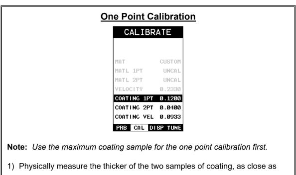
possible to the maximum expected coating measurement range, using a set of calipers or a digital micrometer.
