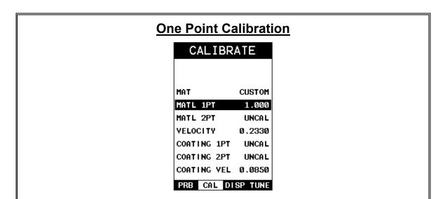
**Note:** Be sure that the probe zero procedure has been performed prior to performing this calibration procedure.
