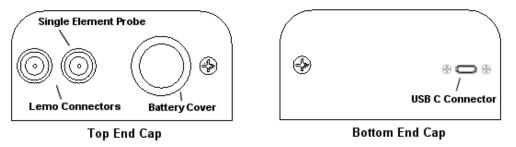
The top & bottom end panels are where all connections are made to the *TI-CMXDL*. The diagram above shows the layout and description of the connectors:
