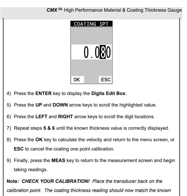
thickness. If the thickness is not correct, repeat the steps above.
