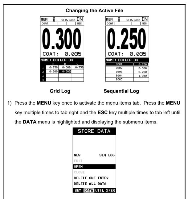
2) Use the **UP** and **DOWN** arrow keys to scroll through the sub menu items until **OPEN** is highlighted.
