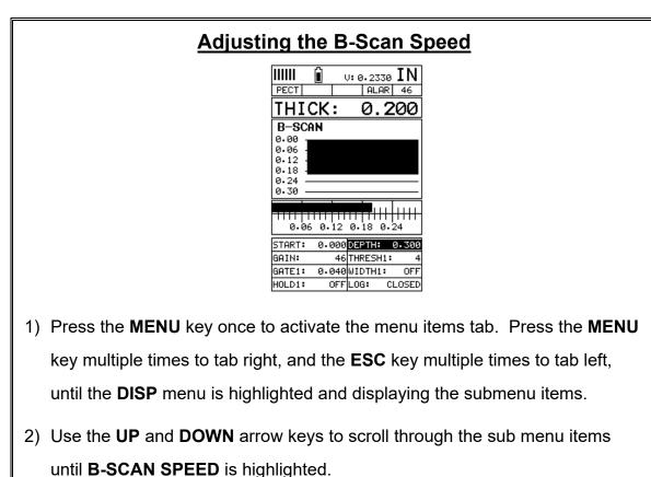
Use the LEFT and RIGHT arrow keys to scroll the speed from 0-10. Note:
