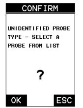
1) Press the **OK** or **ESC** keys to display the factory list of transducer types (by diameter and frequency).
