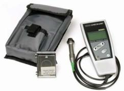
The 3000FX Series is supplied as a complete kit with gauge, ferrous and or non-ferrous zero plate (model dependent), 2 calibration standards, 2 AA batteries, carrying pouch, manual and manufacturer's calibration certificate.
